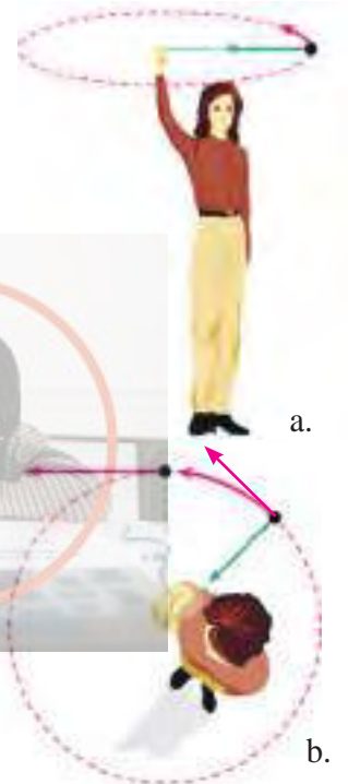
1.2 A stone tied to a string, moving along a circular path and its velocity in tangential direction
